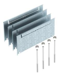
Height compensation set for underfloor boxes UZD250-3 with a construction height of 165 to 220 mm for construction stacking of the UZD to a height of 215-270 mm, consisting of four fall plates, four height adjustment screws and four rotary locks.
