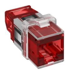
Connection module Cat. 6A (ISO) unshielded, with an RJ45 slot. Including a dust cover, a cable tie, a Keystone fastening frame and mounting instructions. Suitable for installation in the data technology supports of type DTG-2C and DTS-2C, support plate of type MTM 2C and MTM 3C, mounting plate of type MPR2 2C, mounting supports of type MTGE2 2C, MTGE2 15 2C and MTGE2 F 2C.
