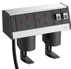
The DB Deskbox ensures a direct supply of the workplace with power, data and multimedia technology and is suitable for fixed attachment to a tabletop. The Deskbox is equipped with a connection cable, which runs out of the profile from below. The housing consists of an anodised, silver-coloured aluminium profile. The Deskboxes can be mounted simply on a tabletop with 2 fastening vices, without damaging the tabletop. Mounting is possible on a tabletop with a thickness of 8 to 40 mm.
