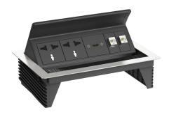
The ready-for-connection, foldable DBK Deskbox ensures a direct supply of the workplace with power, data and multimedia technology. The Deskbox is equipped with a connection cable, which runs out of the profile from below. The visible surface is made of brushed stainless steel and equipped with a brush bar as a cable outlet.
