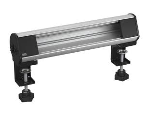
Ready-for-connection Deskbox DBL for the direct supply of workstations with power. With a Wieland GST18® connector and cable outlet at the left side of the profile. Tooless mounting with 2 fastening clamps for tabletop thicknesses of 8 to 40 mm and 40 to 70 mm. The Deskbox is not equipped and can be equipped with up to 5 installation devices of type Modul 45®.
