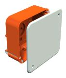
Cavity wall connection box for use in cavity walls with an installation depth of at least 50 mm and a plate thickness of 7-35 mm. With white cover and cover screws. Suitable for installation of standard rails (hat and support rails) for series terminals.
