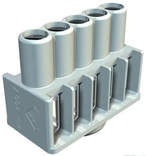
Teminals and screws made of steel, galvanised and transparent-chromated, nominal cross-section  $1 \div 4 \text{ mm}^2$ , rated voltage 400 V, five-pole, with socket terminals, max. connectable cross-sections per terminal:  $4x2.5 \text{ mm}^2$ ,  $5x1.5 \text{ mm}^2$  or  $6x1 \text{ mm}^2$ .
