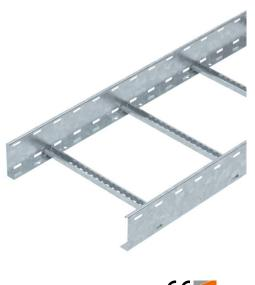
Cable ladder with 110 mm side height with welded C30 profile rungs which are open in an upwards direction. Rolled side rail for reinforcement and as edge protection. Fastening to the bracket takes place using clamps, type LKS 40. The slot dimension of the frame is 16.5 mm and the appropriate clamp clip is type 2056.
