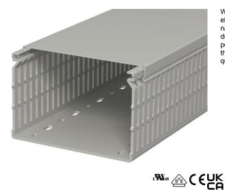
Wiring duct, incl. cover and base perforation, for horizontal and vertical routing of electrical cables in the switchgear cabinet. Designed as a metric duct. The nominal dimension of the system size corresponds to the internal dimension of the duct. Retainers are broken out without tools. The flush-floor routing of cables is possible through predetermined break points. Tapering in the side slots prevents the cables from falling out. Tested to DIN EN 50085-2-3. Special lengths on request.
