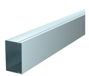
Duct cover and base with base perforation. Equipotential bonding is guaranteed between the cover and the base without any additional aids. The LKM cable duct, type LKM 60100, has been tested for the maintenance of electrical function as a routing system according to DIN 4102 Part 12. Please note the cable types tested in the BSS fire protection systems division! The base contains loop perforation allowing the attachment of the partition.
