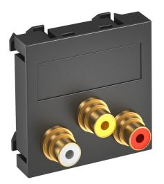
Multimedia support with three cinch connection sockets for audio-video, straight cable outlet, with labelling panel, three cinch sockets (RCA) with soldered connection, colour coding yellow / red / white. Support plate with locking fastening, suitable for horizontal and vertical installation in the system environment.
