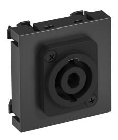
Multimedia support with one Speakon connection socket, straight cable outlet, without labelling panel, Speakon 4-pin socket with screw connection. Support plate with locking fastening, suitable for horizontal and vertical installation in the system environment.
