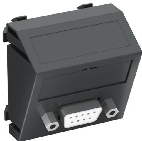
Multimedia support with one D-Sub9 connection socket, slanting cable outlet, with labelling panel, D-Sub9 socket (RS232) with screw connection. Support plate with locking fastening, suitable for horizontal and vertical installation in the system environment.
