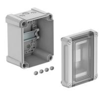
Distribution box for surface mounting, for the current sub-distribution in interior and protected exterior areas, in accordance with IEC 439-3. With pre-mounted 35 mm hat profile rail. IP66 protection type and IK07 protection rating. Transparent cover to screw on, with cut-out.
