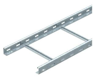
Cable ladder with perforated side rail of side height 45 mm with riveted C profile rungs, open in an upwards direction.
