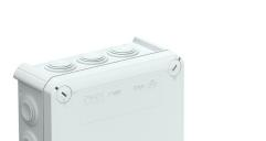
Junction box for the connection of cables and lines indoors and in protected outdoor areas. Rectangular design with plug-in seals to the sides and knock-out entries in the bottom. Suitable for wall and ceiling mounting and on mounting panels. With the option to fasten inside and to mount via the corner domes. Cover with quick lock, sealable. Made from halogen-free and UV-resistant materials.
