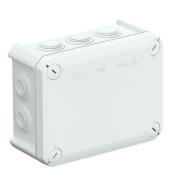
Junction box for the connection of cables and lines indoors and in protected outdoor areas. Rectangular design with plug-in seals to the sides and knock-out entries in the bottom. Suitable for wall and ceiling mounting and on mounting panels. With the option to fasten inside and to mount via the corner domes. Cover with quick lock, sealable. Made from halogen-free materials. Flame-resistant type made from special polypropylene.
