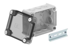
Junction box for the connection of cables and lines indoors and in protected outdoor areas. Rectangular design with plug-in seals to the sides and knock-out entries in the bottom. Suitable for wall and ceiling mounting and on mounting panels. With the option to fasten inside and to mount via the corner domes. High, transparent cover with quick lock, sealable. Made from halogen-free and UV-resistant materials.
