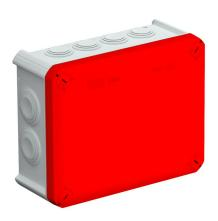
Junction box for the connection of cables and lines indoors and in protected outdoor areas. Rectangular design with plug-in seals to the sides and knock-out entries in the bottom. Suitable for wall and ceiling mounting and on mounting panels. With the option to fasten inside and to mount via the corner domes. Cover with quick lock, sealable. Made from halogen-free and UV-resistant materials.
