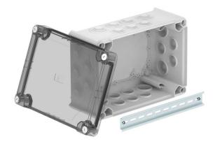
Junction box for the connection of cables indoors and in protected outdoor areas. Rectangular design with plug-in seals. Suitable for wall and ceiling mounting, on mounting panels and threads in the floor. With the option of fastening inside and to mount via the corner domes. High, transparent cover with quick lock, sealable. Made from halogen-free, UV-resistant materials.
