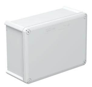
Closed junction box for the connection of cables and lines indoors and in protected outdoor areas. Rectangular design without entries. Suitable for wall and ceiling mounting, on mounting panels and threads in the floor. With the option to fasten inside and to mount via the corner domes. Cover with quick lock, sealable. Made from halogen-free and UV-resistant materials.
