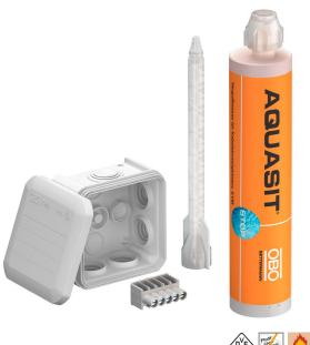
Junction box set with terminal strip for the connection of cables and lines indoors and in outdoor areas exposed to high levels of and long-lasting dampness. Including Aquasit two-component casting compound in a cartridge. Square design with plug-in seals to the sides and knock-out entries in the bottom. Suitable for wall and ceiling mounting and on mounting panels. With the option to fasten inside. With fixed clamping cover. Made from halogen-free materials.
