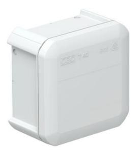
Junction box for the connection of cables and lines indoors and in protected outdoor areas. Square design without entries. Suitable for wall and ceiling mounting and on mounting panels. With the option to fasten inside and to mount via the corner domes. With fixed clamping cover. Made from halogen-free and UV-resistant materials.
