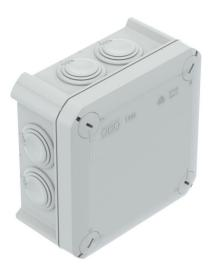
Junction box for the connection of cables and lines indoors and in protected outdoor areas. Square design with plug-in seals to the sides and knock-out entries in the bottom. Suitable for wall and ceiling mounting and on mounting panels. With the option to fasten inside and to mount via the corner domes. Cover with quick lock, sealable. Made from halogen-free materials. Flame-resistant type made from special polypropylene.
