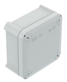
Junction box for the connection of cables and lines indoors and in protected outdoor areas. Square design without entries. Suitable for wall and ceiling mounting and on mounting panels. With the option to fasten inside and to mount via the corner domes. Cover with quick lock, sealable. Made from halogen-free and UVresistant materials.
