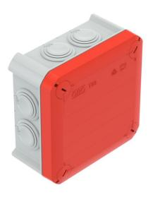
Junction box for the connection of cables and lines indoors and in protected outdoor areas. Square design with plug-in seals to the sides and knock-out entries in the bottom. Suitable for wall and ceiling mounting and on mounting panels. With the option to fasten inside and to mount via the corner domes. Cover with quick lock, sealable. Made from halogen-free and UV-resistant materials.
