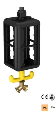
Empty housing with 1 m pipe 1/2" and connection for compressed air hose 13 x 3.5 mm and 2-way distributor 1/2". With suspension lug and grip hook, for the installation of electrical resources, with included partition. Without cover plates.
