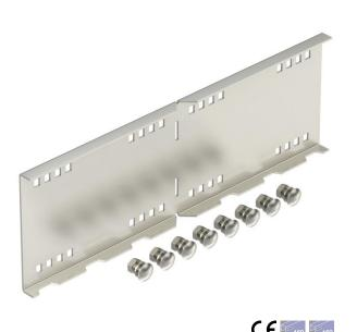
Angle connector for wide span cable trays and ladders with a side height of 160 mm. Including appropriate bolts, washers and nuts.
