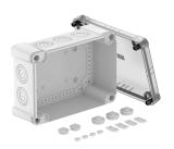
Junction box for the connection of cables and lines indoors and in outdoor areas. Rectangular design with knock-out entries. Suitable for wall and ceiling mounting with the option to fasten outside, inside or to mount via the corner domes. Particularly impact resistant with IK08. Transparent cover with quick lock, sealable. Made from halogen-free and UV-resistant materials.
