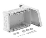
Junction box with terminal strip for the connection of cables and lines indoors and in outdoor areas. Rectangular design with knock-out entries. Suitable for wall and ceiling mounting with the option to fasten outside, inside or to mount via the corner domes. Particularly impact resistant with IK09. Cover with quick lock, sealable. Made from halogen-free and UV-resistant materials.
