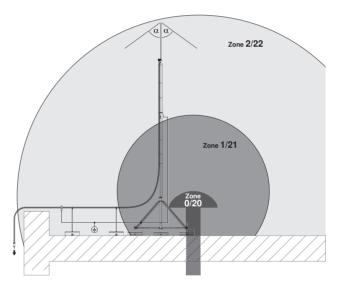
Example of the installation of the isCon<sup>®</sup> Pro+ system in the Ex zones of a potentially explosive area
